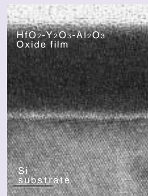
Fig.3: Structural characterization by TEM. An amorphous structure was confirmed in the area indicated the red circle in Fig.2.
