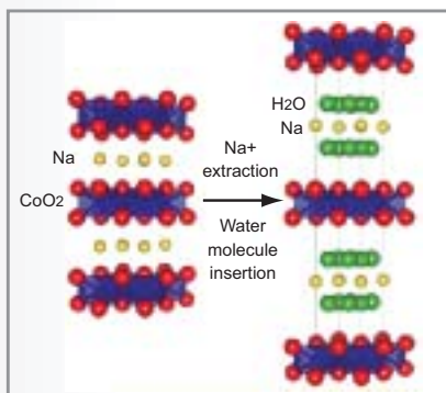
Fig.1 Crystallographic structure of precursor (Na 0.7 CoO 2 (left) and newly-discovered Na 0.35 CoO 2 ·1.3H 2 O with superconductivity.
