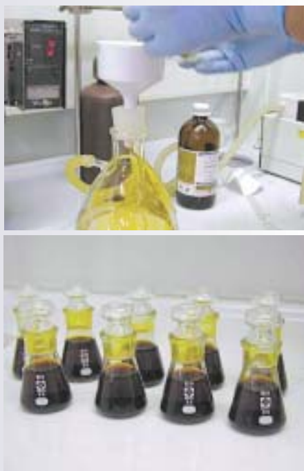
Fig.1 Synthesis of \text{Na}_x\text{CoO}_2 \cdot y\text{H}_2\text{O} (Top, filtration treatment; bottom, bromine treatment).
