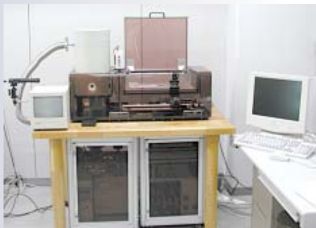
Fig. 1 View of the SQUID magnetic microscope.
