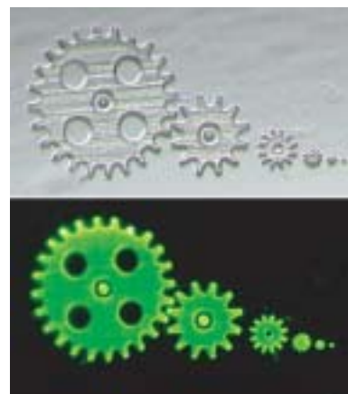
Fig. 3 Micro gears fabricated by laser polymerization technique (diameter: 160 \mu\text{m} to 5 \mu\text{m} ).
