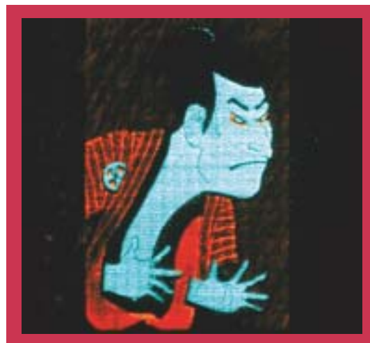
Fig. 4 Fluorescence image of micro array of resin dots containing multiple species of organic molecules (340 \mu\text{m} x 530 \mu\text{m} ).
