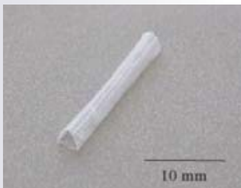
Fig. 2 Chitosan tube for use in nerve regeneration.
