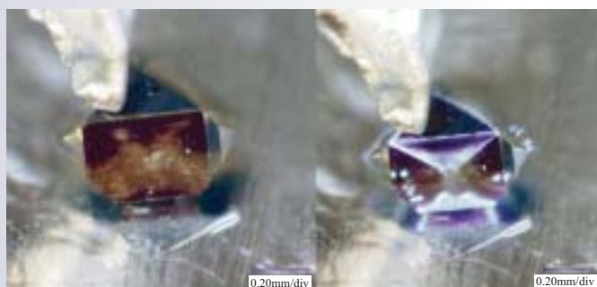
Fig. 1 Light emissions from cBN single crystal with spontaneously-formed p-n domain. (Left) before impressing voltage, (right) after impressing voltage.
