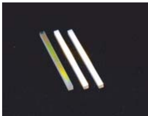
Fig. Examples of new wavelength conversion device (rod-shaped) using MgO-doped stoichiometric \text{LiTaO}_3 crystals. Standard size: 2 x 2 x 35L mm.
