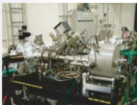
Fig. 3 Photoelectron microscope in beamline hatch.
