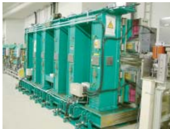
Fig. 1 Revolver switching-type undulator X-ray source.
