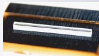
Wavelength conversion device of periodically poled stoichiometric LiTaO 3 . Nd:YAG laser beam (1064 nm wavelength) can be converted into a laser beam of wavelength in a range from 1.4 to 4 microns.
