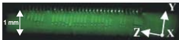
Fig. 2 Image of real-time observation of periodic twin fabrication (period: 125 \mu\text{m} ).
