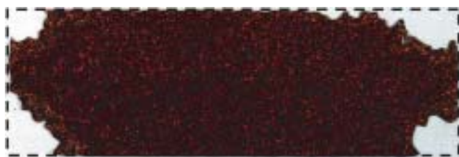
Fig. 1 Appearance of Fe-1%Al alloy exposed for 2 years at Miyakojima (broken line shows original shape of test piece).
