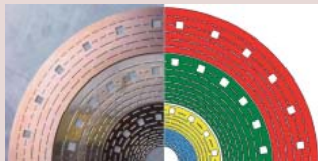
Comparison of the Bitter-disks used in the previous magnet and new magnet. Disk in the right side is the new disk.
