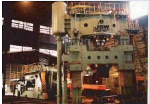
Fig. 2: Large-scale press at Japan Steel Works, Ltd. used in test production of UFG plate.
