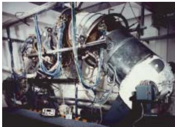
Fig: Bending creep test of actual piping at MPA. (Figure provided by Prof. Maile.)
