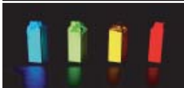
Fig. 2 Top: Nitrooxide fluorphor developed by NIMS. Middle and bottom: Fluorescent powder developed by NIMS.
