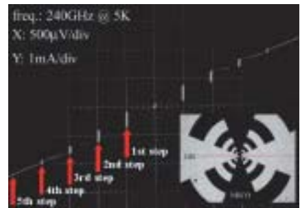
Fig. 3 Current-voltage characteristic of fabricated grain boundary junction at 5 K in a microwave field of 0.24 THz. Microwave induced Shapiro steps are indicated by red arrow. The insert shows the optical microscopic image of junction with wiband planar logarithmic-periodic antenna.
