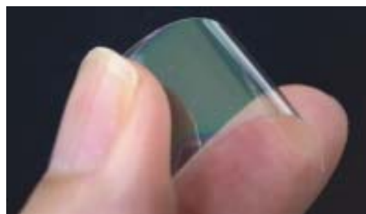
Fig. 1 Photocatalyst TiO_2 thin film fabricated on a PET resin film without heating.
