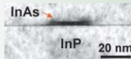
Fig. 1 TEM image of cross section of an InAs quantum dot fabricated on InP (001) substrate.
