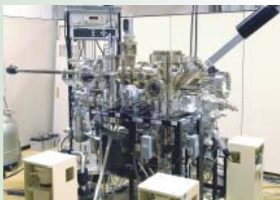
Fig. 1 Ultra-high vacuum multiple-scanning-probe microscope.
