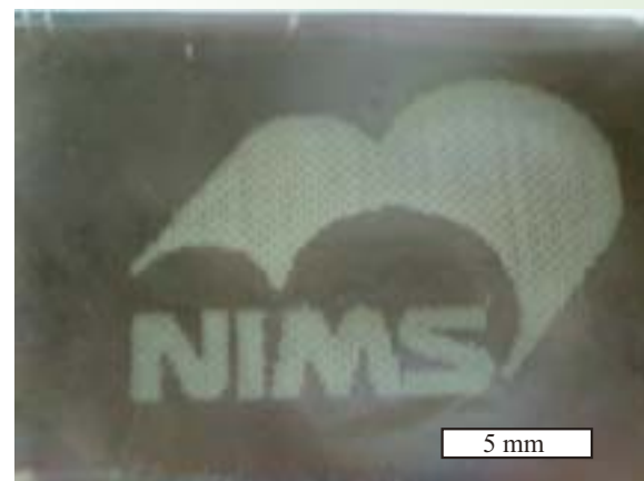
Fig. 2 Logo mark stands out distinctly using the photocatalytic effect of a \text{TiO}_2 film formed on an unheated glass substrate.
