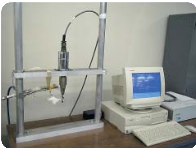
Fig. 2 Ultrasonic fatigue tester (20 kHz).
