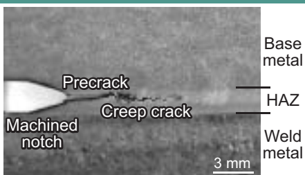
Fig. 1 Results of creep crack growth test using CT specimen of welded joint (growth of Type IV crack).
