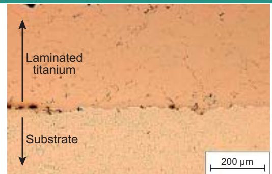
Fig. 2 Photograph of the cross-section of laminated titanium on a metal substrate fabricated by the warm spray process.
