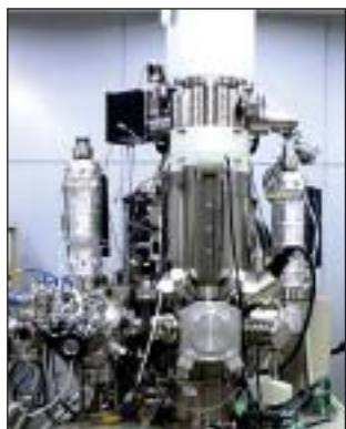
Fig. 1 Appearance of ultra-high vacuum, aberration-corrected STEM.
