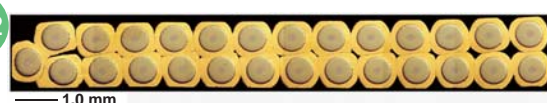
A Rutherford cable made by weaving together 27 Nb 3 Al superconducting wires. The cable was compression molded to a high fill ratio of 87%, and is capable of carrying a large current of more than 25,000 A in liquid helium (4.2 K). The cable was trial-manufactured in the summer of 2007 in joint work with the Fermilab.
