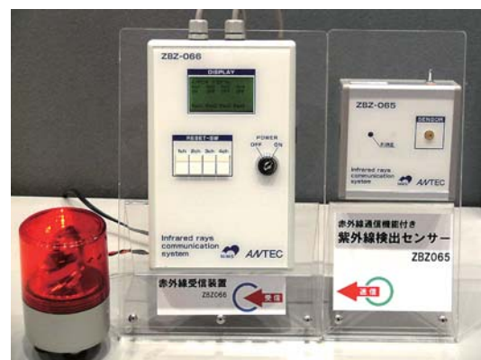
General view of the diamond fire detection system developed using the diamond deep UV sensor. From the right, the system comprises a sensing section, which contains the fire sensor, an alarm control section, and a warning lamp.
