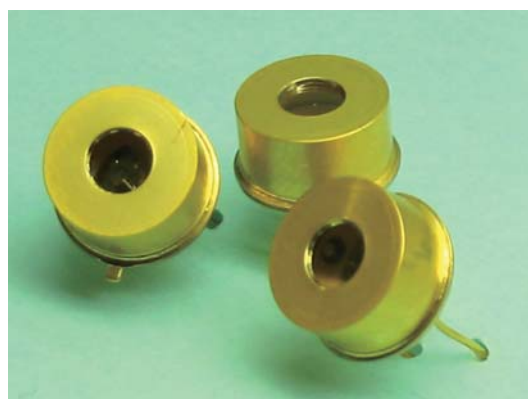
Photograph of the diamond fire sensor. The sensor device is sealed in an airtight package 9 mm in diameter and 5 mm high.
