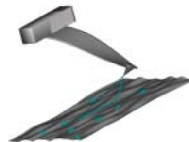
Fig. 2 Horizontal nanomechanical measurement method. The figure shows the observation of nanomechanical events when a molecule is elongated parallel to the substrate. The blue area is a macromolecule such as a protein. The mechanical properties of the molecule are measured while it is stretched along the substrate surface. The substrate is surface-modified silicon, glass, or the like.
