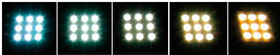
Fig. 2 White LEDs using developed red, green, and yellow phosphors.
