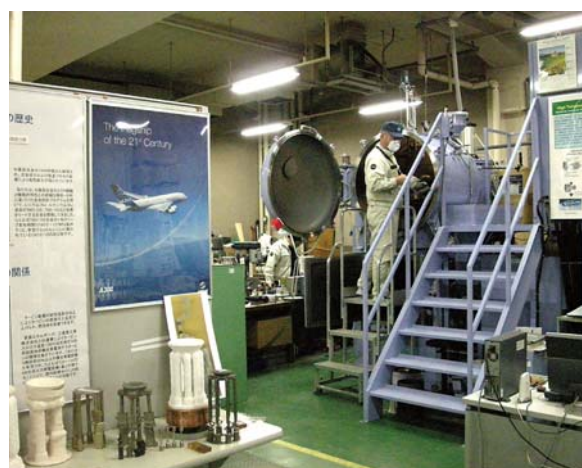
Casting of a Ni-base single crystal alloy using a directionally solidified casting furnace. As shown at the right, after molten alloy is cast into a special mold in the vacuum furnace, a single crystal material is produced by the withdrawal method. Various types of test specimens have been prepared from this cast material.
