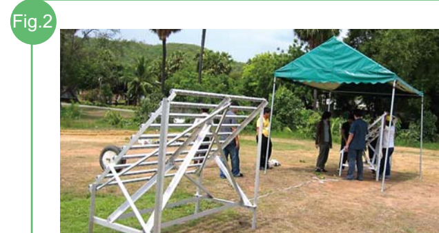
Preparations for the exposure test in Thailand (exposure site: Pattaya). Front: Direct exposure rack, rear: shielded exposure rack.
