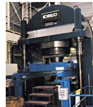
NIMS’s 30,000t high pressure synthesis device. This device enables large capacity high pressure synthesis experiments at pressures in the range up to 10GPa.
