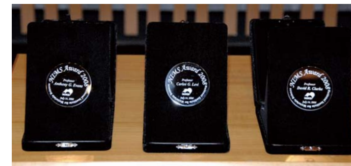
NIMS Award 2008 Medals Made from Ni-free High Nitrogen Austenitic Stainless Steel by NIMS
