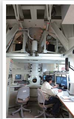
High Voltage Electron Microscopy Station: Dual ion beam interfaced high voltage TEM
