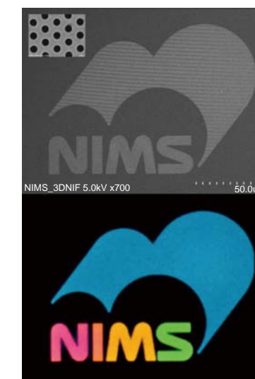
Fig.2 Surface plasmon color filter fabricated in this research. Top: Scanning electron microscope image, bottom: transmitted light image.
