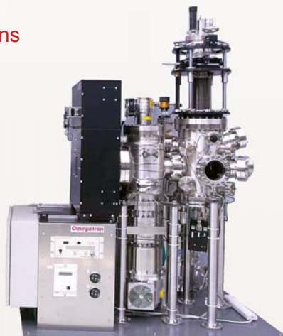
Fig. 2 Prototype of the spin-polarized low-energy ion scattering spectroscopy device He + ion beam: polarization 25%, energy 10eV – 2keV, current <100nA Analyzer: angle-resolved, hemispherical, electrostatic, theta and phi rotation
