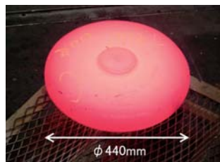
Fig. 3 Forged pancake manufactured through C&W process for real components (440mm dia.).
