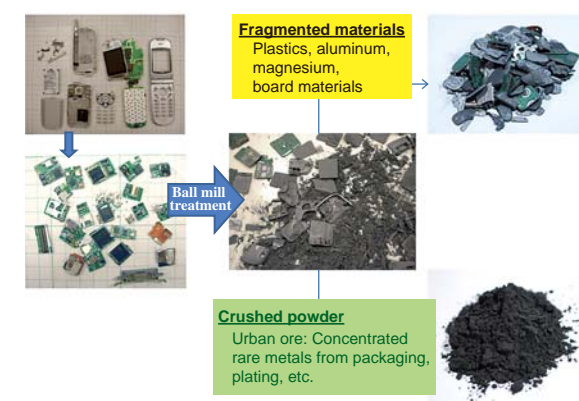
Fig.1 Outline of treatment process Used cell phones (left) which have been roughly crushed to a size suitable for charging into the ball mill are treated by the ball mill (center). Plastics, aluminum, board materials, etc. remain in fragment form (upper right). LSI chips, parts, etc. packaged on the boards are selectively separated and crushed, and are concentrated as powder "urban ore."
