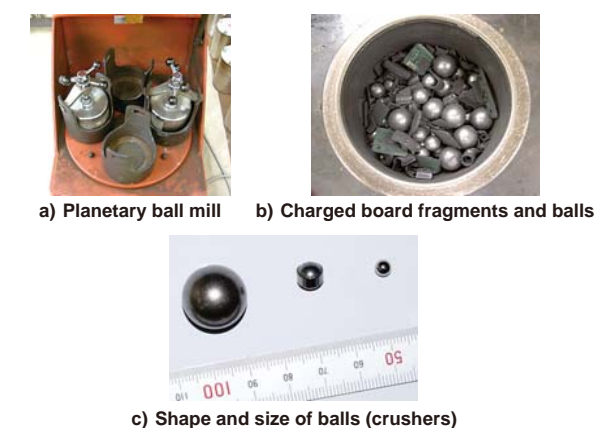
Fig.2 a) Ball mill actually used (planetary ball mill) b) Roughly crushed used cell phones are placed into a container containing balls made of a hard material. The container is set in a planetary ball mill device (a), and the container itself rotates (self-revolution) while revolving around the central axis of the device.
