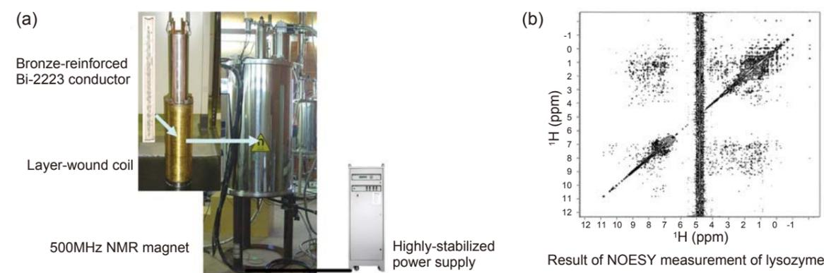
Fig. NMR magnet containing a high  $T_c$  superconducting coil and an example of NMR measurement.
