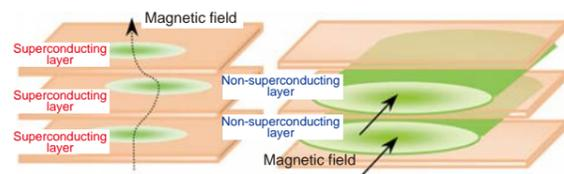
Fig.1 Schematic diagram of the vortices in an oxide high temperature superconductor, showing the case where the magnetic field is perpendicular to the superconducting layer (left) and parallel to the superconducting layer (right).
