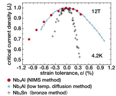
Fig. 1 Comparison of strain tolerance in superconducting wires developed for a fusion reactor
