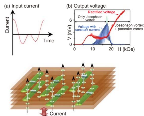
Fig.3 Coexistence of pancake vortices and Josephson vortices. (a) shows a time-asymmetrical input current, and (b) is the rectified output voltage.
