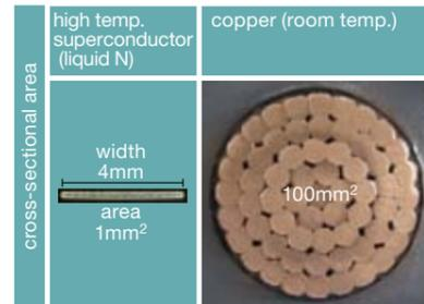
Cross-sectional area of conductors required for each 100 A of transmission current, assuming that the bismuth oxide high- $T_c$  superconductor tape wire is operated at 50% of its critical current (about 200 A at the temperature of liquid nitrogen)
