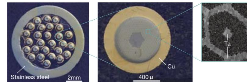
Fig. 2 Cross section of a prototype Nb<sub>3</sub>Al-based CIC conductor
