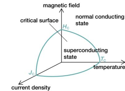
Fig. 3 Critical surface of a superconductor
