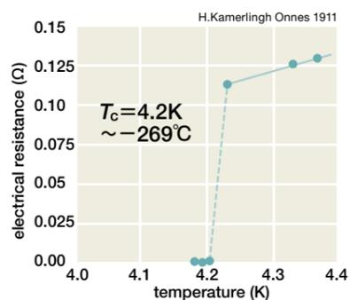
Fig. 1 At 4.2 K the resistance of mercury drops abruptly and disappears, as stated in Onnes' article of 1911
