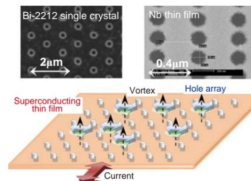
Fig.2 Vortices move in a hole array in superconductor thin films (see photos) when driven by an electrical current.
