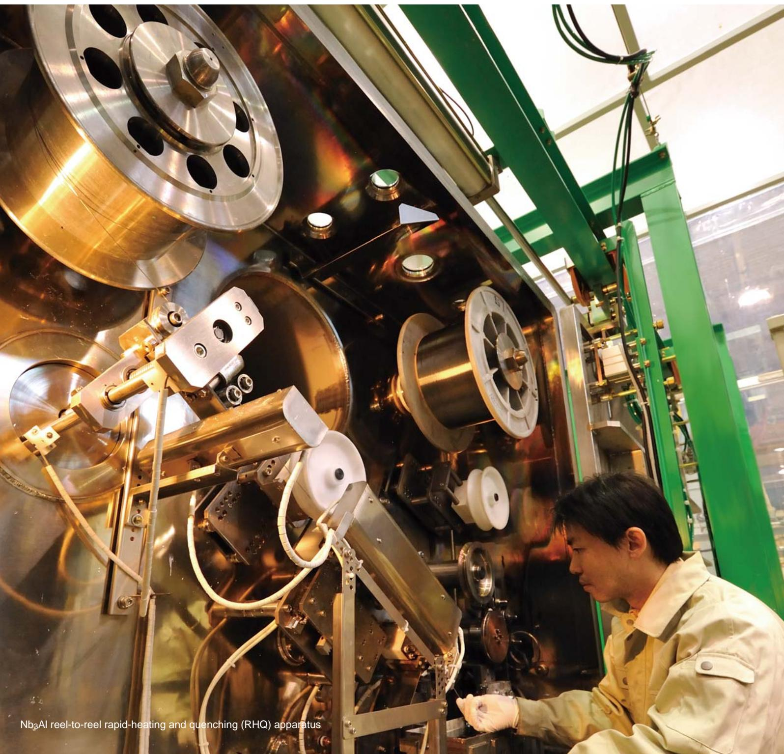
$\text{Nb}_3\text{Al}$  reel-to-reel rapid-heating and quenching (RHQ) apparatus
