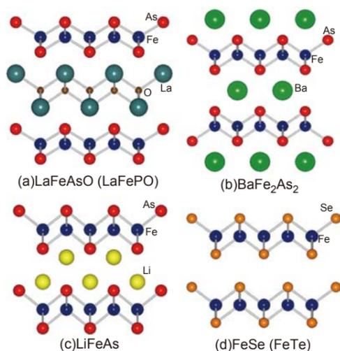
Fig.1 Crystal structures of various Fe-based superconductors. The respective  $T_c$  are (a) 55K, (b) 38K, and (c) 18K. The  $T_c$  of (d) FeSe is 13K, but this increases to 37K under pressure.
