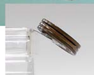
Fig. 4 The polyimide/SMA actuator lifting three coins weighing 4.5g each.
