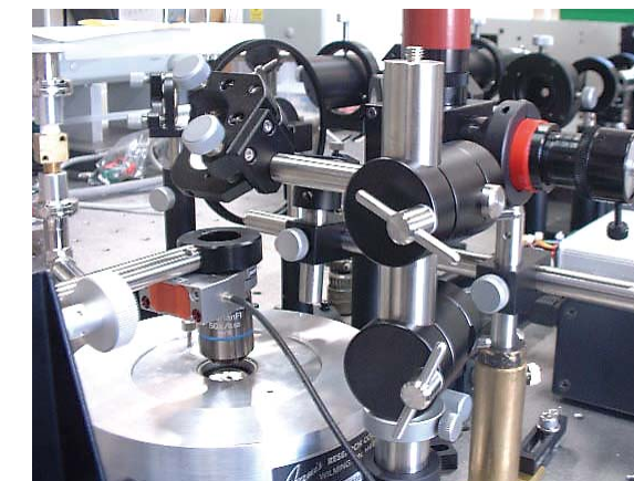
Fig.2 Photo of the NIMS micro-spectroscopy. The specimen is placed between the glass windows of the vacuum cooler under the objective lens of the microscope in the foreground of the photo.
