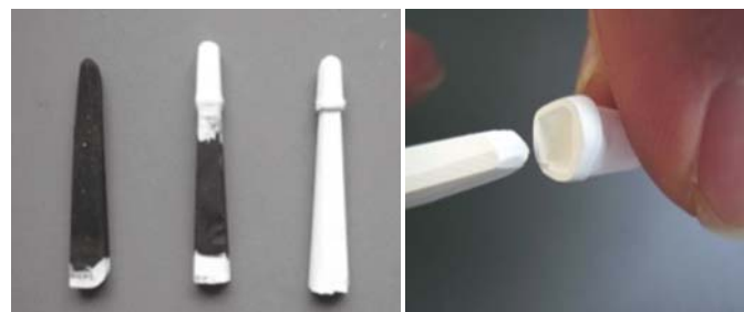
Fig.1 Example in direct shaping of ceramics by electrophoretic deposition using conductive polymer-coated non-conductive ceramic substrates. This technique can be utilized for fabricating various shape-controlled ceramics, such as dental crown.
