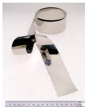
Fig. Intermetallic Ni 3 Al foil fabricated by cold rolling (thickness: 23μm).
