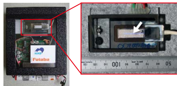
Fig.2 Far UV light source with drive by dry cell batteries; the enlarged view shows the prototype light-emitting device. The blue line shown by the arrow is the light output part. A weak visible light component (400nm), which is emitted together with the intense far UV, appears as bluish-white.
