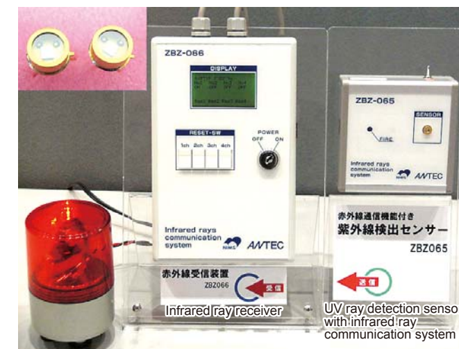
Fig. 2 Fire detection system using diamond solar-blind UV sensor.
