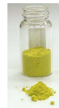
Fig.3 Visible light-responsive photocatalyst. Silver phosphate powder (left). Wavelength dependence of light absorption capacity (left axis) and apparent quantum yield in oxygen generation test (right axis) of Ag_3PO_4 .
