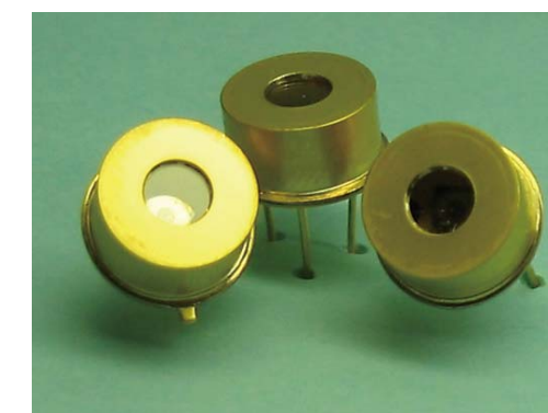
Fig.3 Appearance of diamond deep-UV sensor. This sensor is the result of integrated research and development from the sensor material to the device. By using this sensor, it is possible to detect potential danger in a service environment. Detection helps to guarantee the safety of structural materials.
