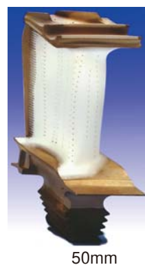
Fig.1 Single crystal turbine blade for use in large-scale jet engines.
