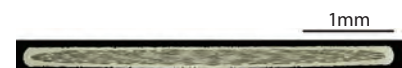
Fig. 5 NIMS Bi-based high T_c superconducting wire. Multi-filaments of (Bi,Pb) _2 Sr _2 Ca _2 Cu _3 O _x superconductor are dispersed in a silver and silver alloy matrix
