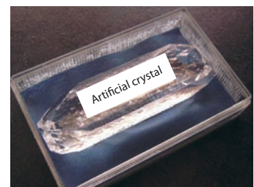
Fig. 2 Artificial crystal quartz grown by hydrothermal synthesis process.
