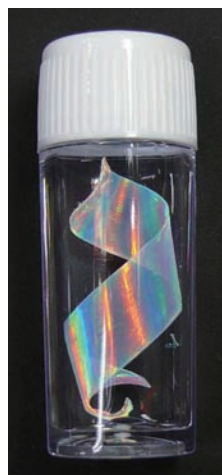
Fig. 2 Artificial opal film fixed by a polymer gel matrix (colloidal crystal gel). The rainbow coloration is caused by Bragg reflection of light.
