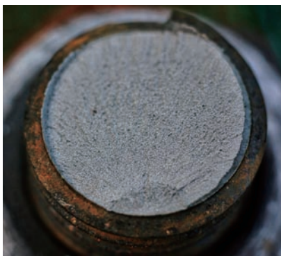
Fig. 1 Example of a bolt that suffered delayed fracture when exposed outdoor in Tsukuba, Japan. Its hydrogen embrittlement susceptibility is increased by increasing the strength of bolts from that of products in practical use.
