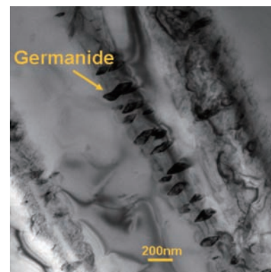
Fig. 2 Novel precipitate formed in the developed alloys.
