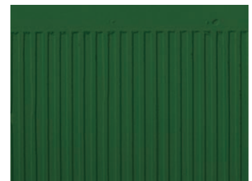
Fig. 3 Nonlinear optical device for polarity control which generates green light by wavelength conversion.
