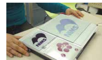
Fig. 3. Colors produced by metallo-supramolecular polymers
