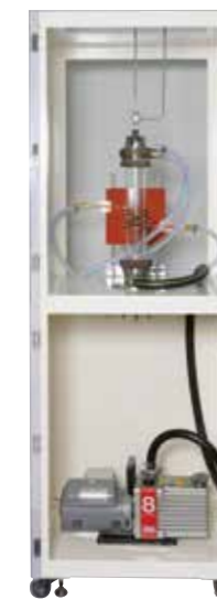
Photo 2. MOVPE Apparatus No. 1 displayed at the Akasaki Institute, Nagoya University
