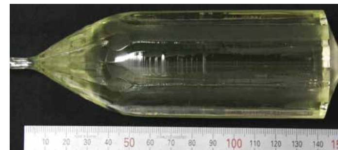
TSLAG single crystal that was developed at NIMS and is in production by Fujikura Ltd.
