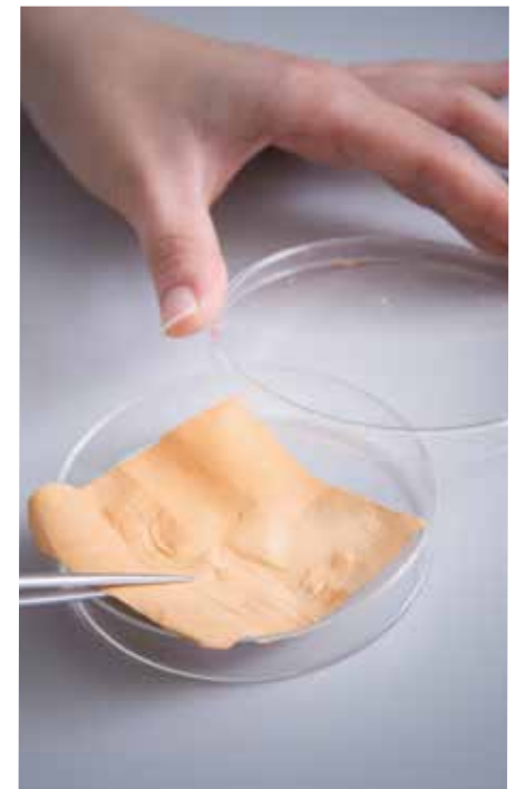
A nanofiber sheet Ebara developed. It looks like ordinary nonwoven fabric, but it contains anticancer drugs and magnetic particles.
