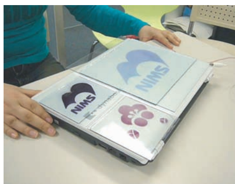
Fig. 3 Display device 10 inches in size using hybrid polymer
