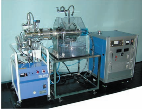
Photo 2. Fabrication apparatus type 3 for metal nano-particles. Almost all kinds of metallic nano-particles can be fabricated except for rare-earth metals or high-melting metals.
