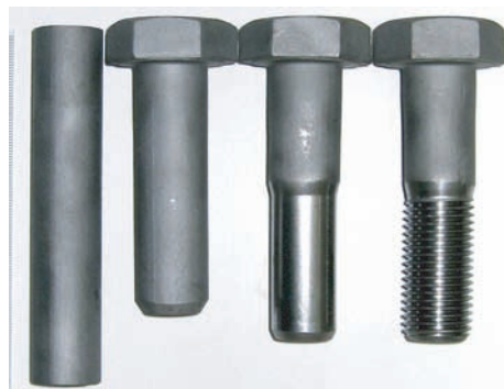
Fig. 5 Photo of the formation process of a M22 bolt with the 1800 MPa-class prototype steel developed at NIMS that is superior in delayed fracture tolerance. The head part was formed in hot pressing, since the prototype steel was harder than the usual steel even after the softening process, and it was difficult to form the hexagonal head part in cold pressing. The thread part was formed in cold forging 2) .
