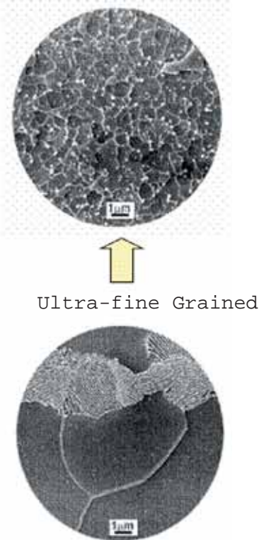
Fig.1 The microstructure of ultra-fine grained steel.
