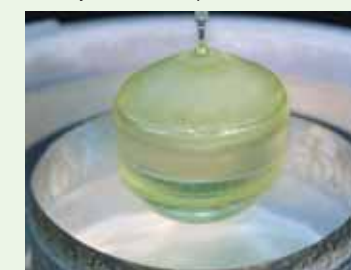
Growth of single crystal under defectcontrol by double crucible method developed in NIMS.
