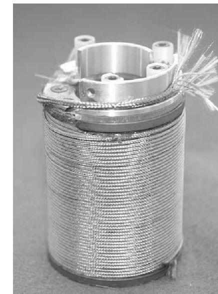
Fig.4 Example of MgB 2 solenoid coil (Outer diameter: 48mm, Inner diameter: 30mm, Height: 50mm. Number of turns: 459).
