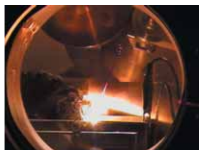
Fig.3 Continuous rapid heating and quenching apparatus.
