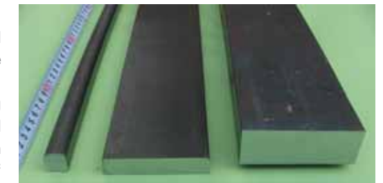
Fig.3 Various forms of ultra-fine grained steel.
