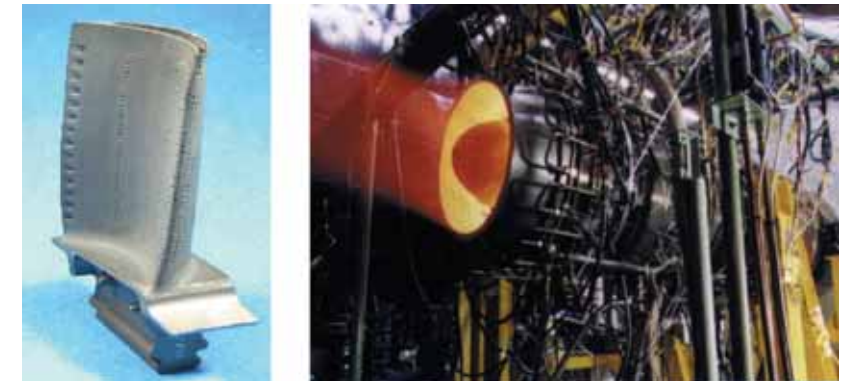
Fig.3 A turbine blade made of TMS-138 and the supersonic engine test on the test bed.
