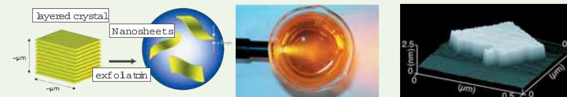
Schematic explanation of exfoliation of a layered crystal into nanosheets, a photograph of a suspension of \text{MnO}_2 nanosheets, and an AFM image of a \text{Ca}_2\text{Nb}_3\text{O}_{10} nanosheet.
